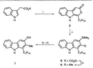
Scheme 1 Reagents and conditions: i,  $(C_7H_{15}CO)_2O$ , BF<sub>3</sub>·Et<sub>2</sub>O, 75%; ii, Me<sub>3</sub>SiC=CCO<sub>2</sub>Et, PhBr, reflux, 74%; iii, LiAlH<sub>4</sub>, dioxane, reflux, 99%; iv, Hg(OAc)<sub>2</sub>, AcOH; v, BH<sub>3</sub>·THF; vi, H<sub>2</sub>O<sub>2</sub>, aq. NaOH; vii, aq. HCl
